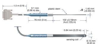
$\textbf{NOTE:} + \boldsymbol{\Phi}$  is designated as that flux passing through the coil, into the side with the Lake Shore logo on the probe handle
